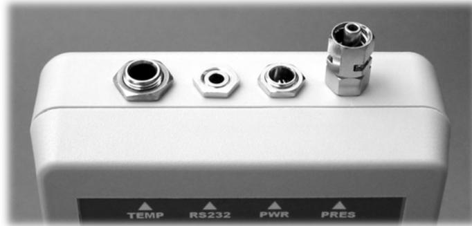
**PRESSURE INPUT** – Male luer lock connector is used for the pressure input.
