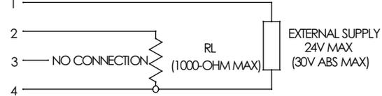
TYPICAL WIRING OF ANALOG VOLTAGE OUTPUT 0 - 10V
