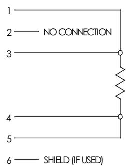
TYPICAL WIRING OF 1000-OHM 3 WIRE RTD
