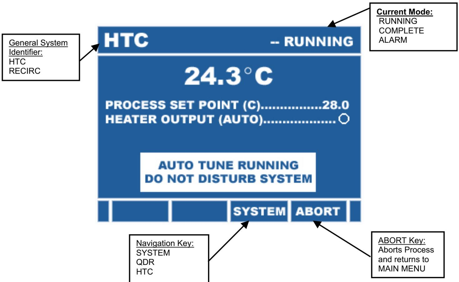
During this procedure, the system will run a test sequence to determine basic system characteristics. After completing this sequence, the appropriate tuning values will be calculated and automatically inserted into the PROP BAND, RESET and RATE parameters.
