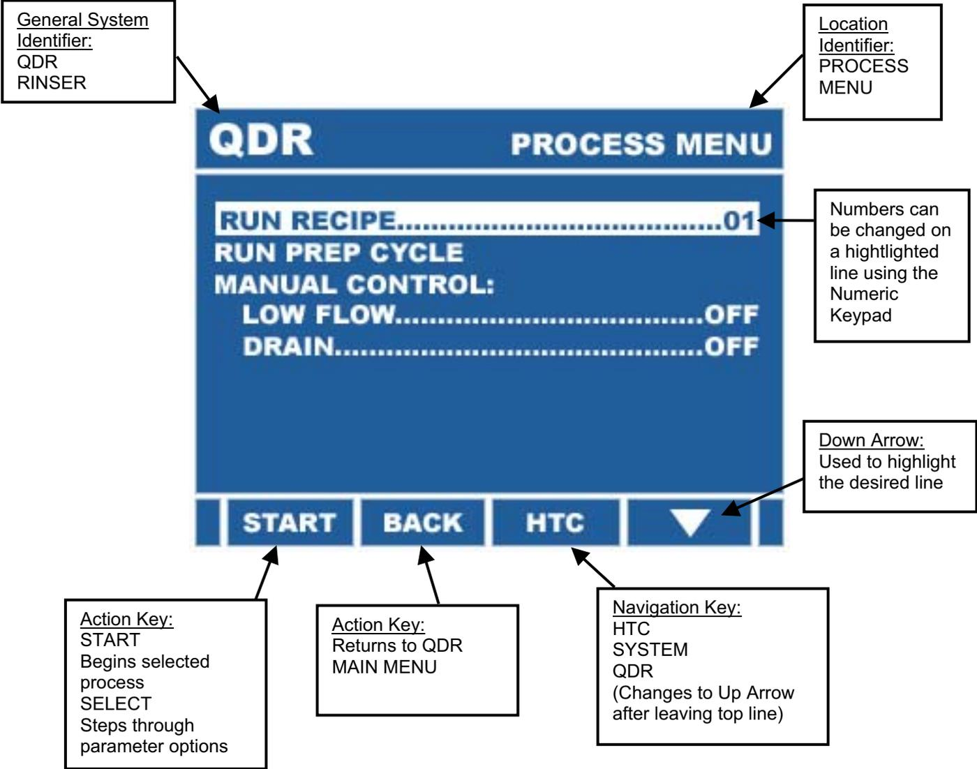
**RUN RECIPE        xx** – This line allows the user to select the recipe that is to be run using the Numeric Keypad and then begin the run using the START key.
