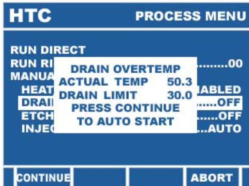
Again press the CONTINUE key. This will place the unit in the AUTO START mode. In this mode the function will run in the background, continuously monitoring the process temperature and automatically starting the drain when the temperature falls below the DRAIN SETPOINT.
