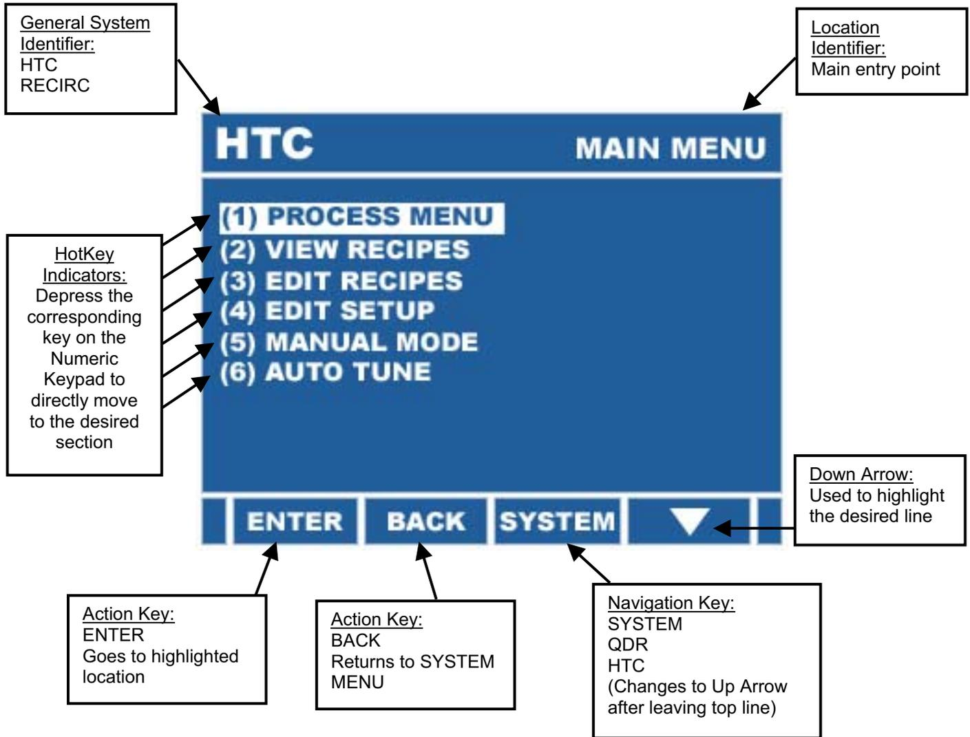
\* Several types of Temperature Controllers are configurable under this section. However, all references and examples will use the most common setting of HTC (High Temperature Controller). The differences between this and the other settings only relates to the labeling of the screens and the specific functions that are available.
