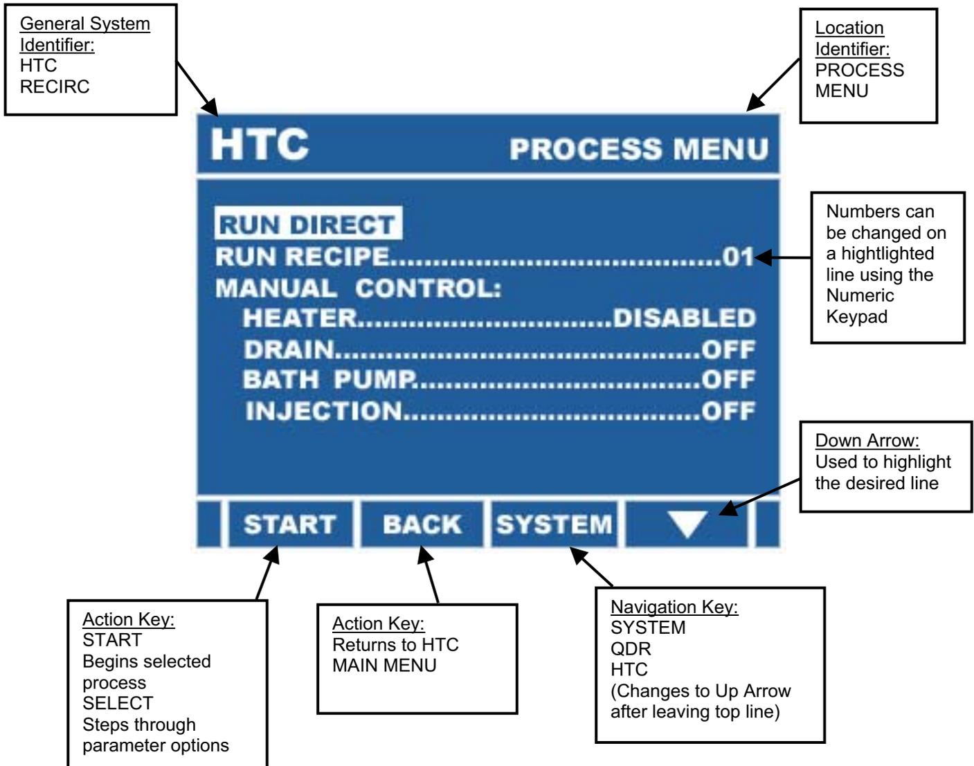
**RUN DIRECT** – This line allows the user to enter the run screen for the HTC. In this mode direct and full control is available. The setting in recipe 00 are used. Also, a Quick Set Timer feature allows the timer to be set with the Numeric Keypad without returning to the RECIPE EDIT screen.
