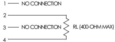
TYPICAL WIRING OF ANALOG CURRENT OUTPUT (BOOST) 0 - 20mA
