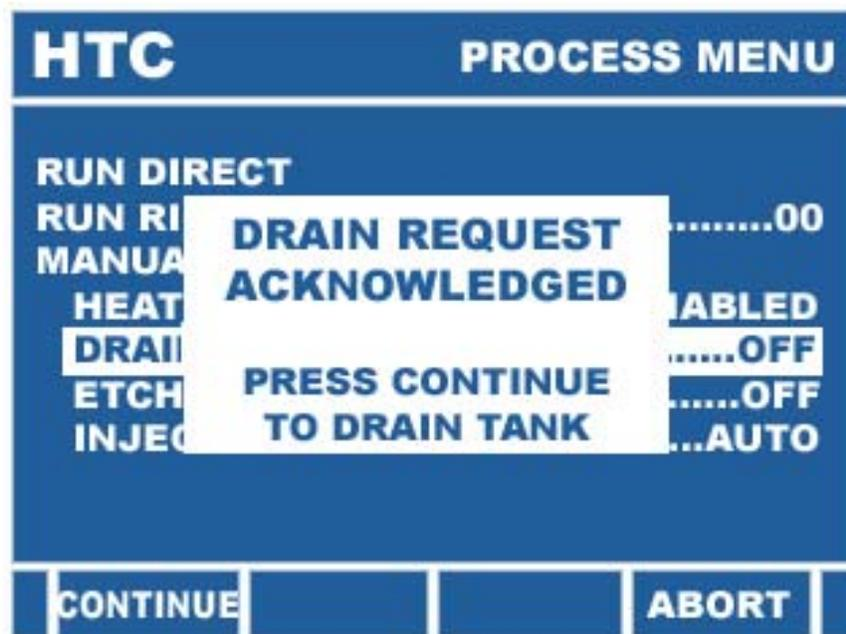
Press the CONTINUE key to proceed. At this point the Heater, Etch Pump, Inject feature and process timer are turned off and locked out.
