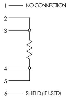
TYPICAL WIRING OF 100-OHM 3 WIRE RTD
