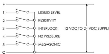
TYPICAL WIRING OF REMOTE INPUTS FOR USE WITH INTERNAL POWER SUPPLY
