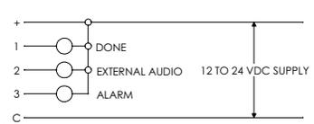
DETAIL OF TYPICAL RELAY OUTPUT
