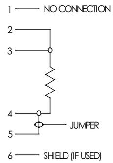
TYPICAL WIRING OF 1000-OHM 4 WIRE RTD
