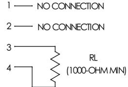
TYPICAL WIRING OF OUTPUTS (OPEN COLLECTOR DRIVER)
