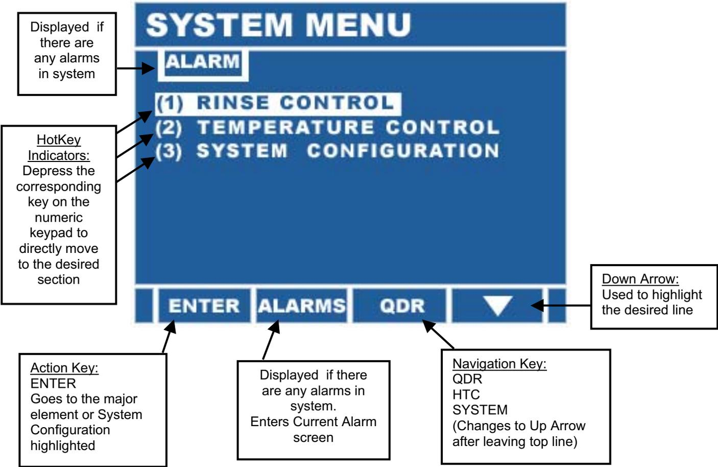
The sections of the unit are entered from this menu in one of several ways. In the first, the ARROW keys may be used to highlight the desired section and the ENTER key is then used to go to that section.
